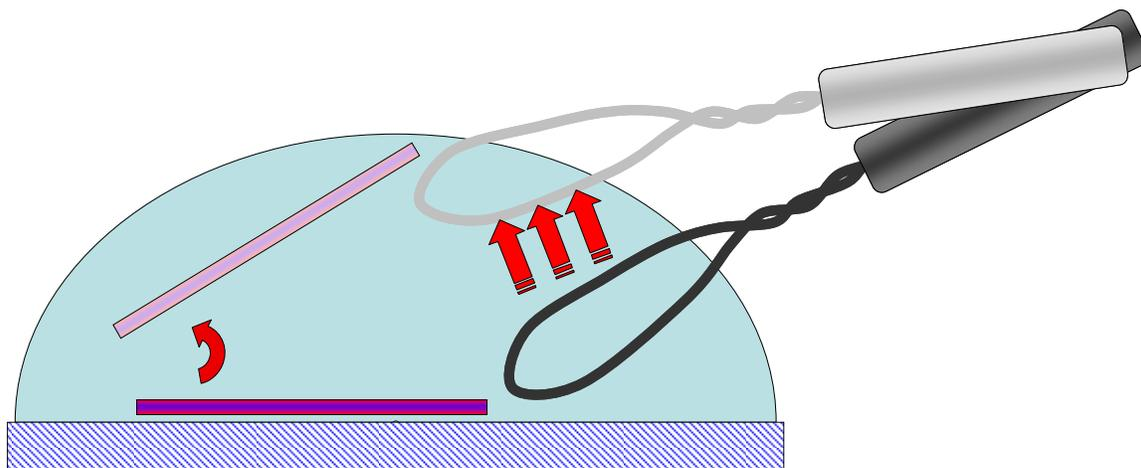
After the crystal is properly positioned, quickly place the loop under the crystal and align the principal axis of the loop with that of the crystal.
