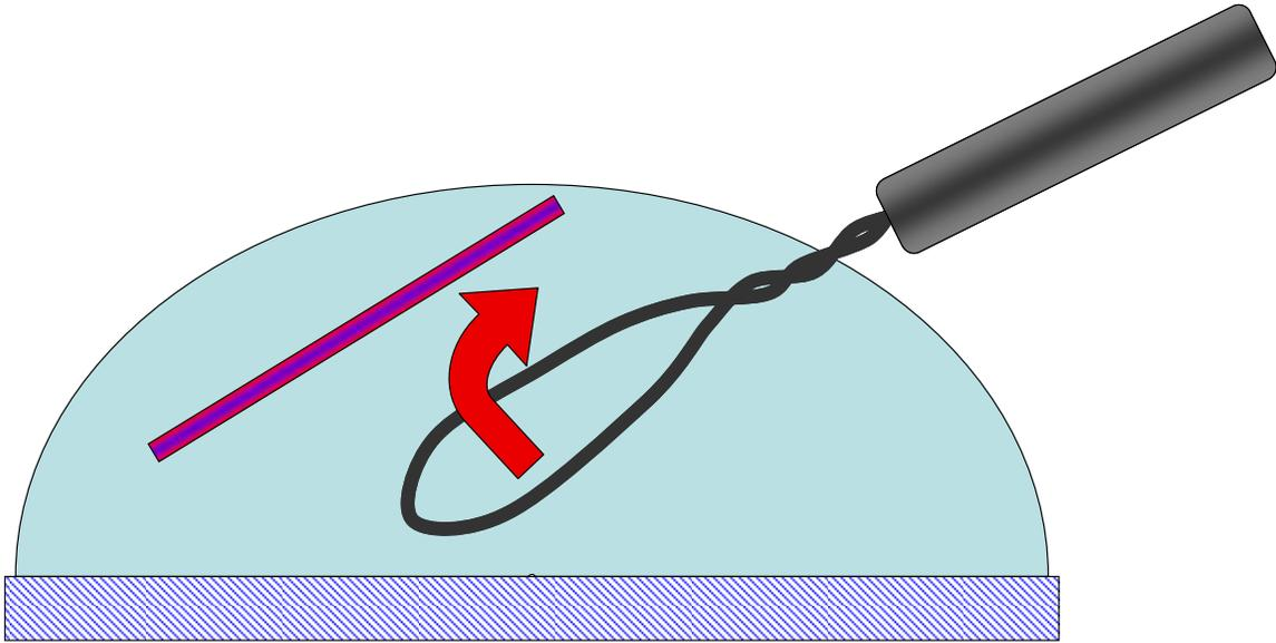
With one smooth motion lift the crystal up and back (towards the stem of the loop) so that the loop drags the crystal out of the mother liquor along its principal axis. Take care to avoid pushing the crystal upwards through the surface of the drop – that is an almost certain way to break the needle. In other terms, let the loop do the work of breaking the surface tension, not the crystal.
